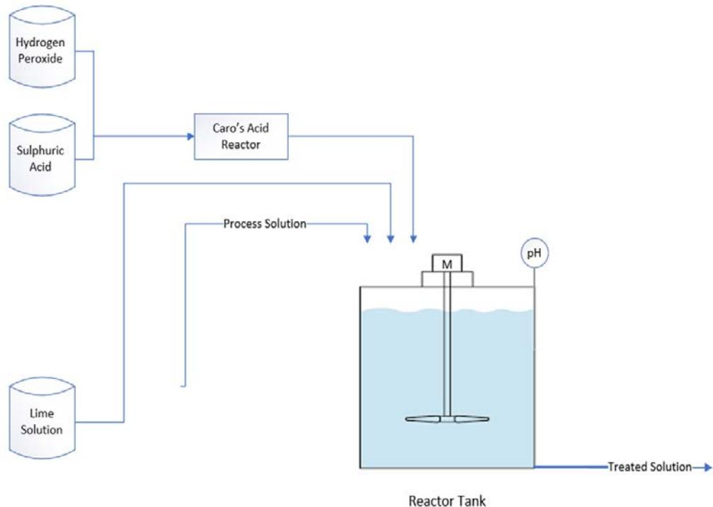
The hydrogen peroxide, sulphuric acid, and lime solution would be piped into the reactor tank from vendor supplied totes.
