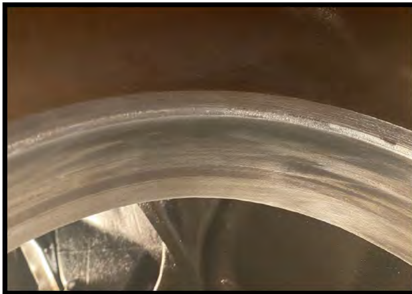
Figure 28 - #5 Left Lower Liner Fit
