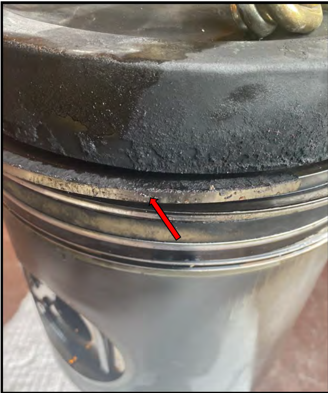
Figure 7 - #4 Right Piston - Ring with carbon
