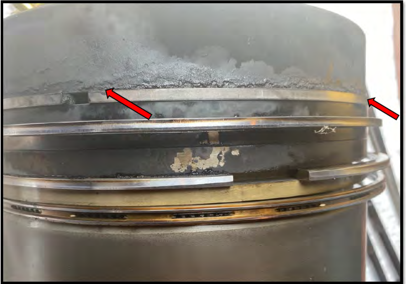
Figure 24 - Piston #5 Left - Top ring seized and flaking
