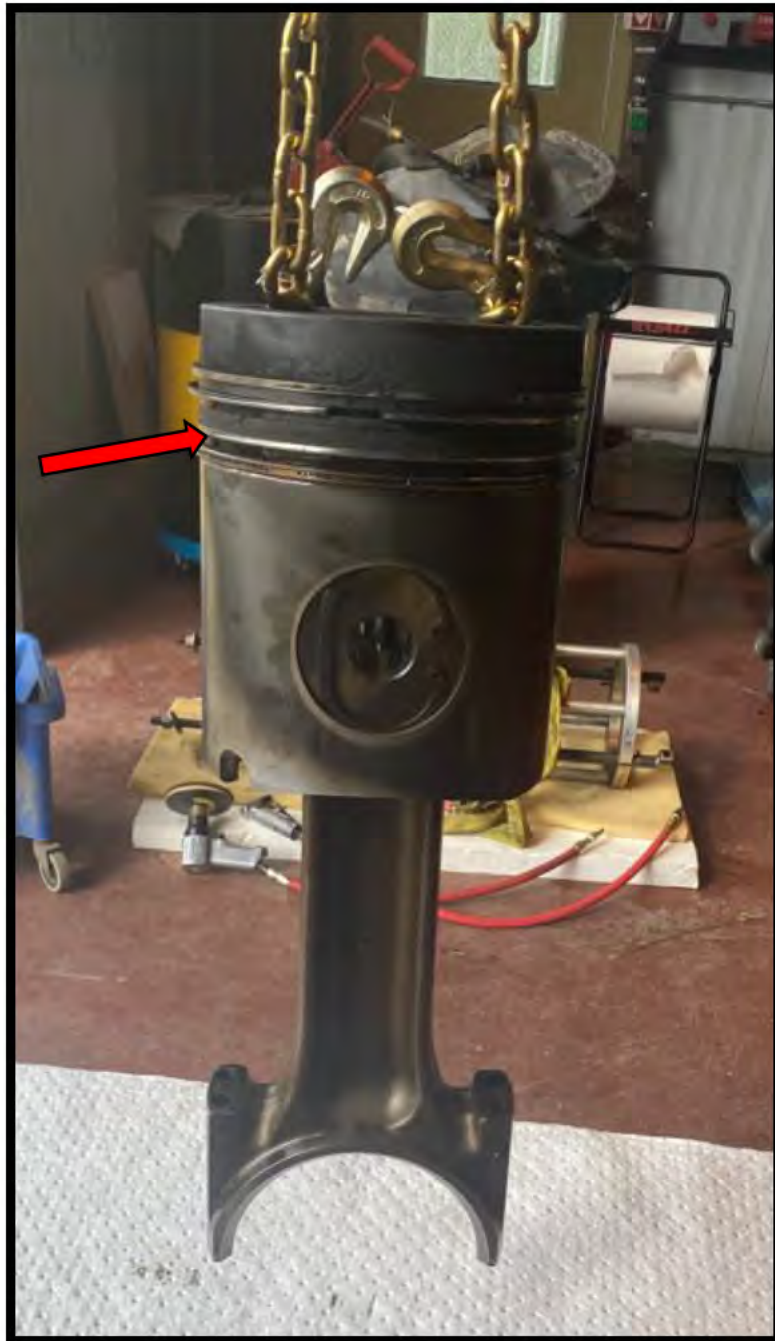
Figure 6- #4 Right Piston - Seized Third Ring
