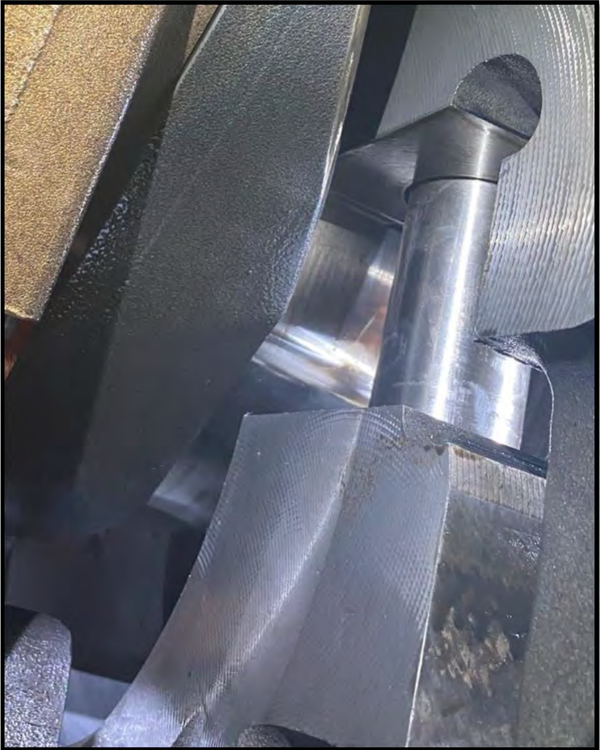
Figure 18- Crankshaft #4 Main Journal
