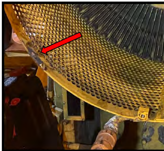
Figure 2- Front Dampener Guard - 7 Broken Tabs
