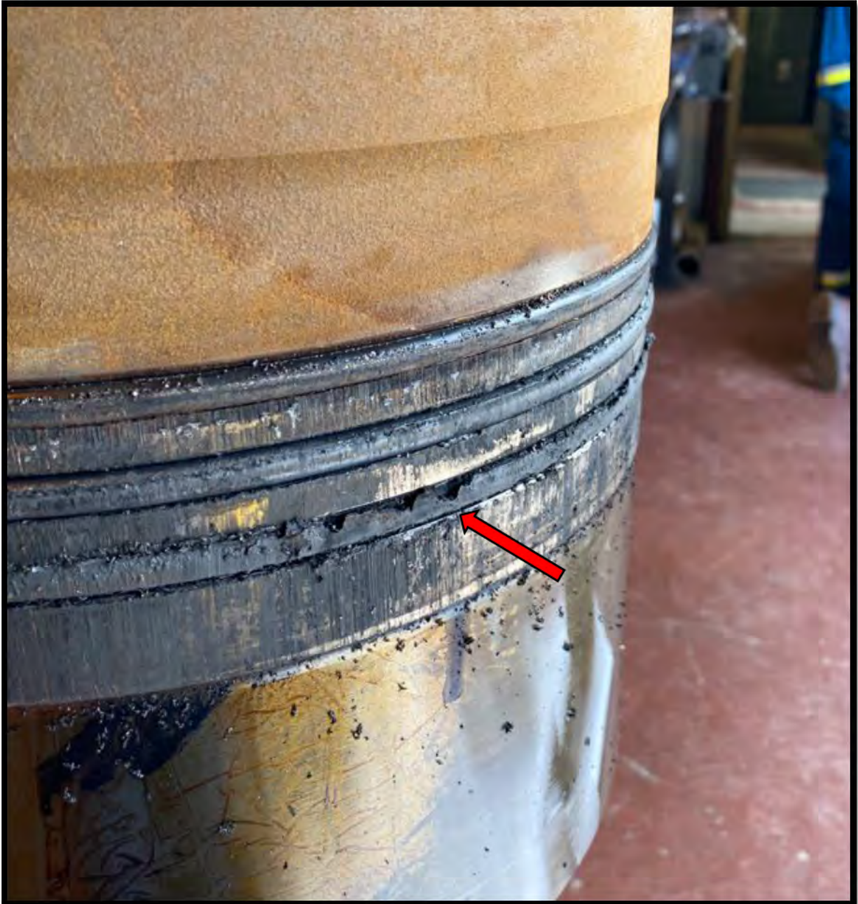
Figure 12- #4 Right Liner O-rings
