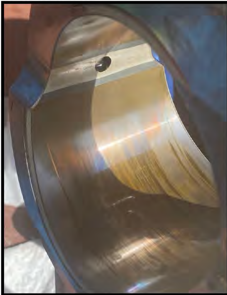
Figure 21 - #4 Right Connecting Rod Bushing
