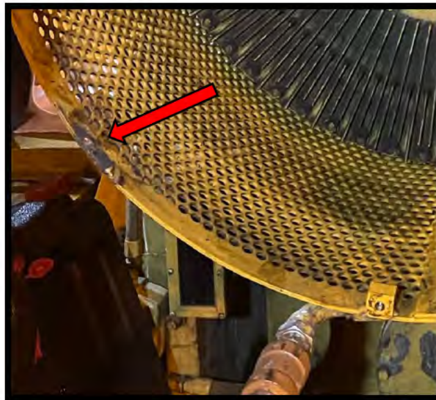
Figure 2- Front Dampener Guard - 7 Broken Tabs
