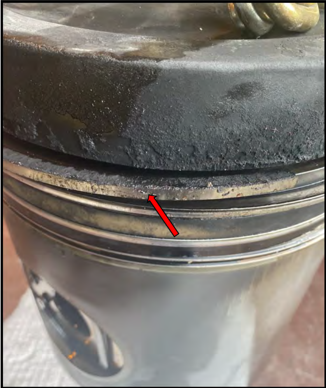
Figure 7 - #4 Right Piston - Ring with carbon
