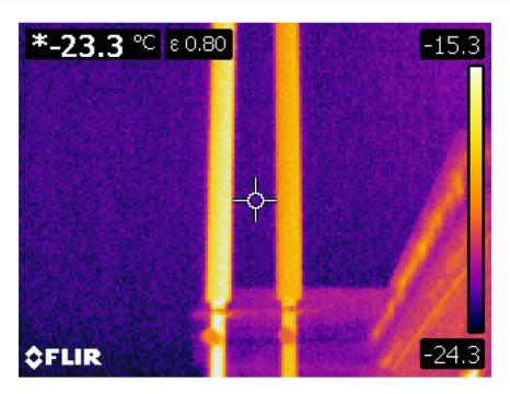
This information would be reviewed, along with the recorded ground temperatures from the datalogger, to verify that the thermopiles are extracting heat from the ground and operating as designed.
