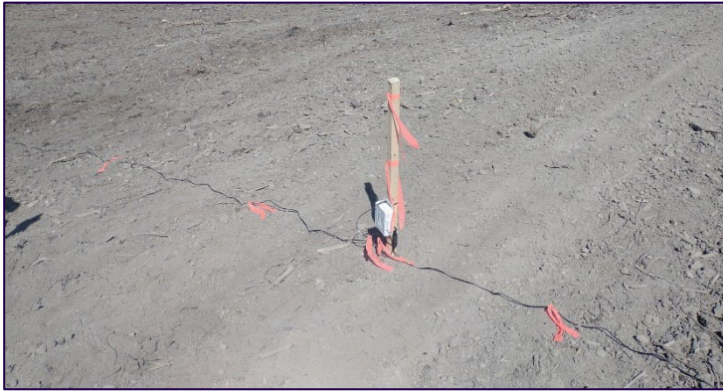
PHOTO 4 HOBO LOGGER CONNECTED TO MOISTURE SENSORS
