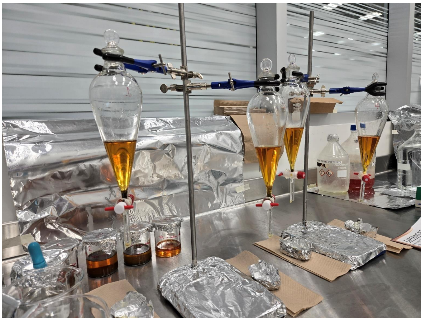
Figure 10. Microplastic Extraction - Density Separation with Sodium Iodide ( \text{NaI}_{\text{aq}} )
