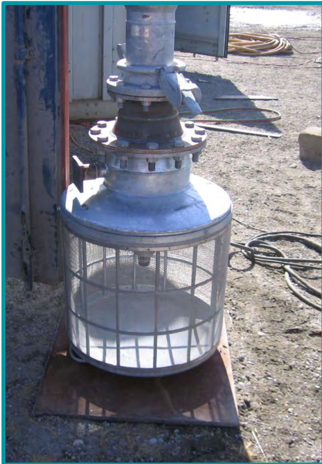
2.3.1-02 A very large fish screen for a high velocity 8" to 10" pump.
