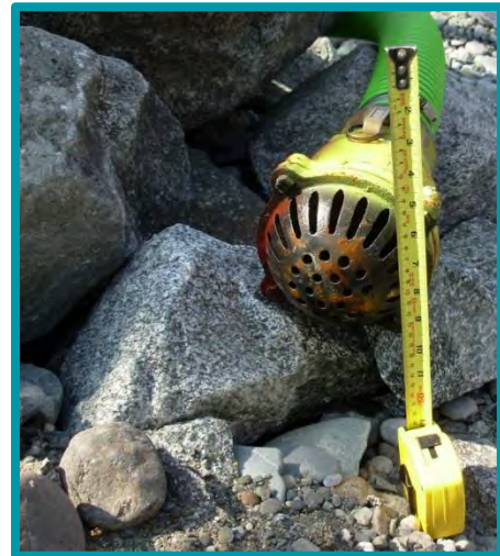
2.3.1-03 An example of a fish screen with holes that are too large.
