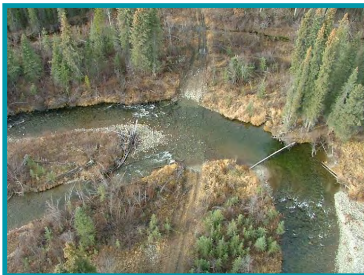
3.4-01 This type of stream fording is a thing of the past in Yukon, and never should have reached this state. There obviously have been multiple fordings over the course of years, leaving permanent marks in a fish-bearing stream. A temporary bridge should have been installed.
