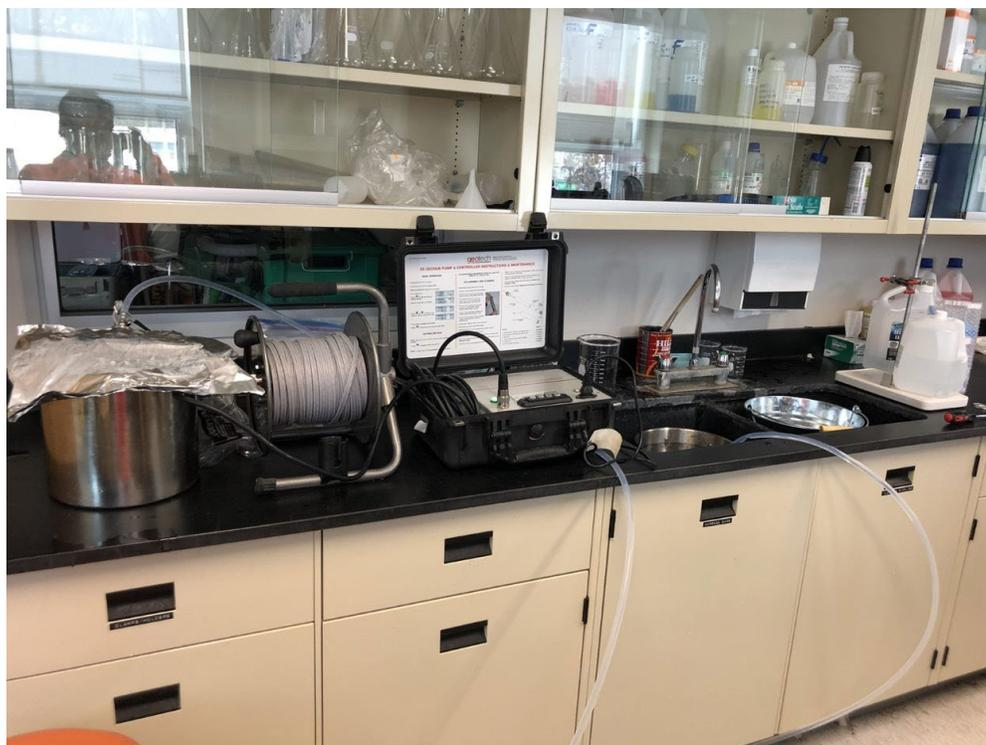
**Photo 3-7: Filter Blank Processing with 100L Deionized Water in WRB's Laboratory**
