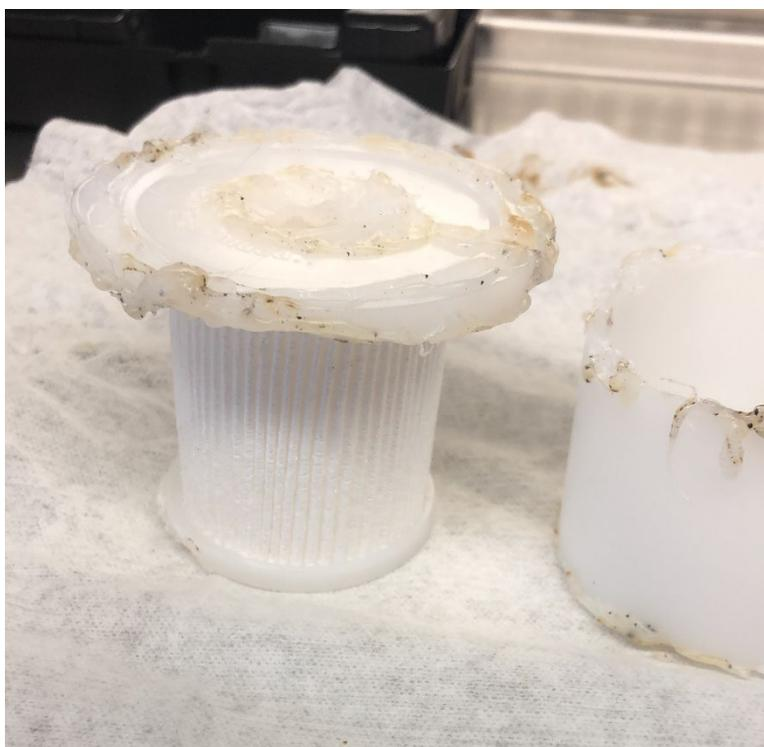
**Photo 3-8: Filter Removed from Plastic Casing using Hot Blade**
