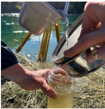
Figure 2. Back rinsing sieve to collect the sediment into sample jars.
