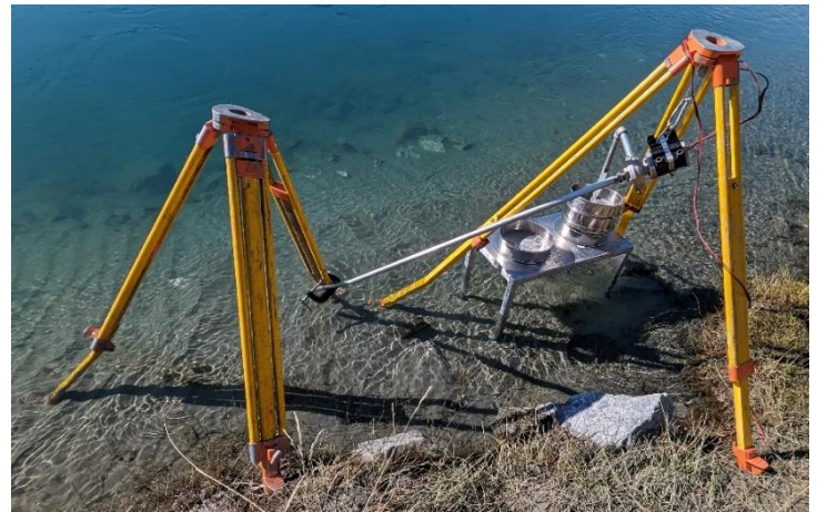
Figure 1. The sampling equipment set up in the Yukon River. The pump is suspended from two wooden tripods, positioning the intake on the upstream side and the outlet over the filter sieve, downstream of the intake to avoid recirculating water.
