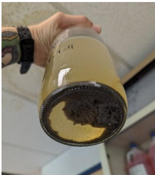
Figure 3. Sediment sent for analysis representing several thousand litres.
