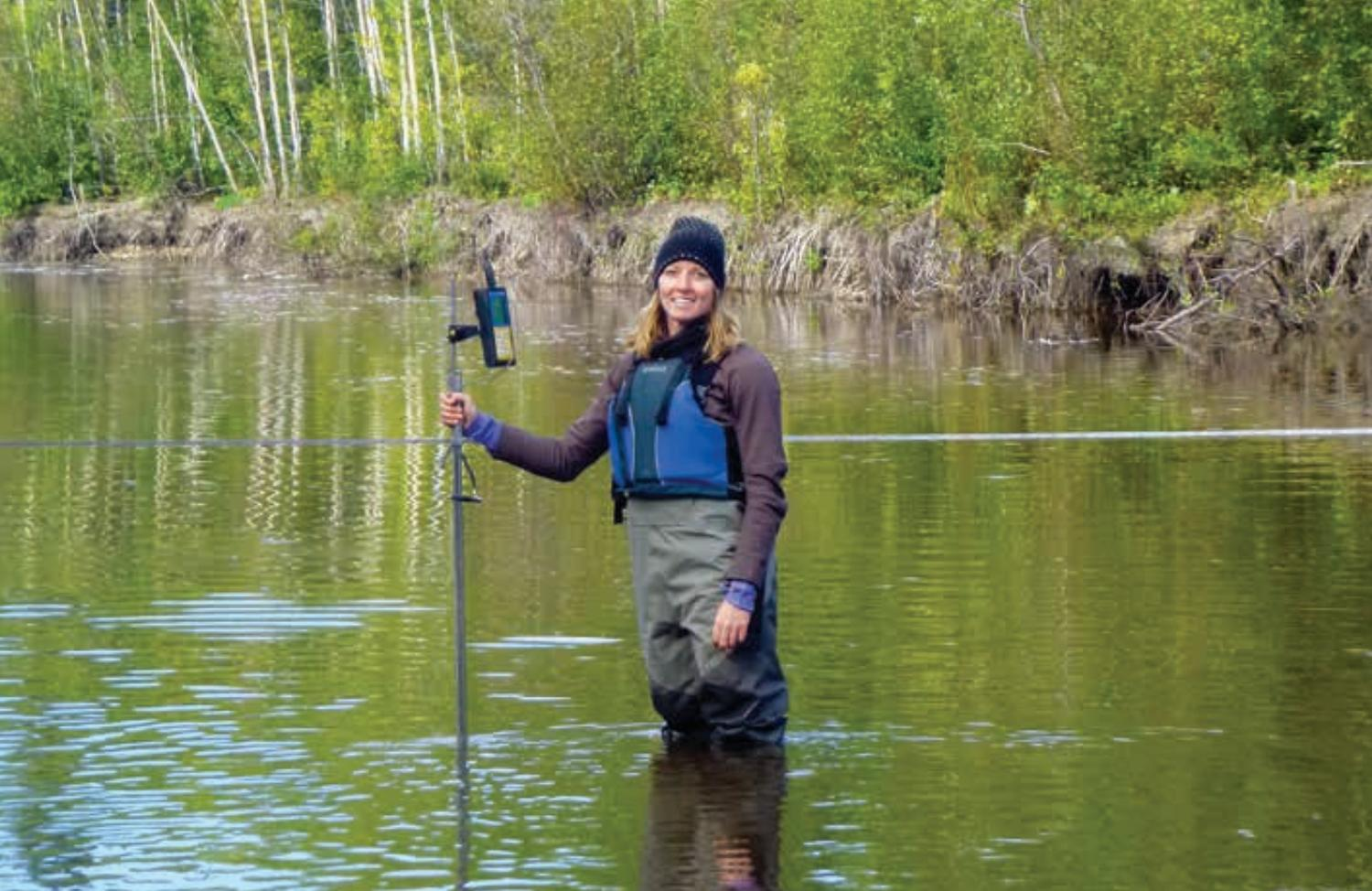
Water discharge measurement on Dalglish Creek in the Peel River watershed
