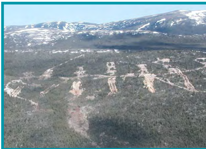
3.12-01 Large-scale trenching. In Yukon, many projects are multifaceted, include construction of access roads or trails, and are never very far from a watercourse. Planning and the application of preferred practices are key to erosion and sediment control.
