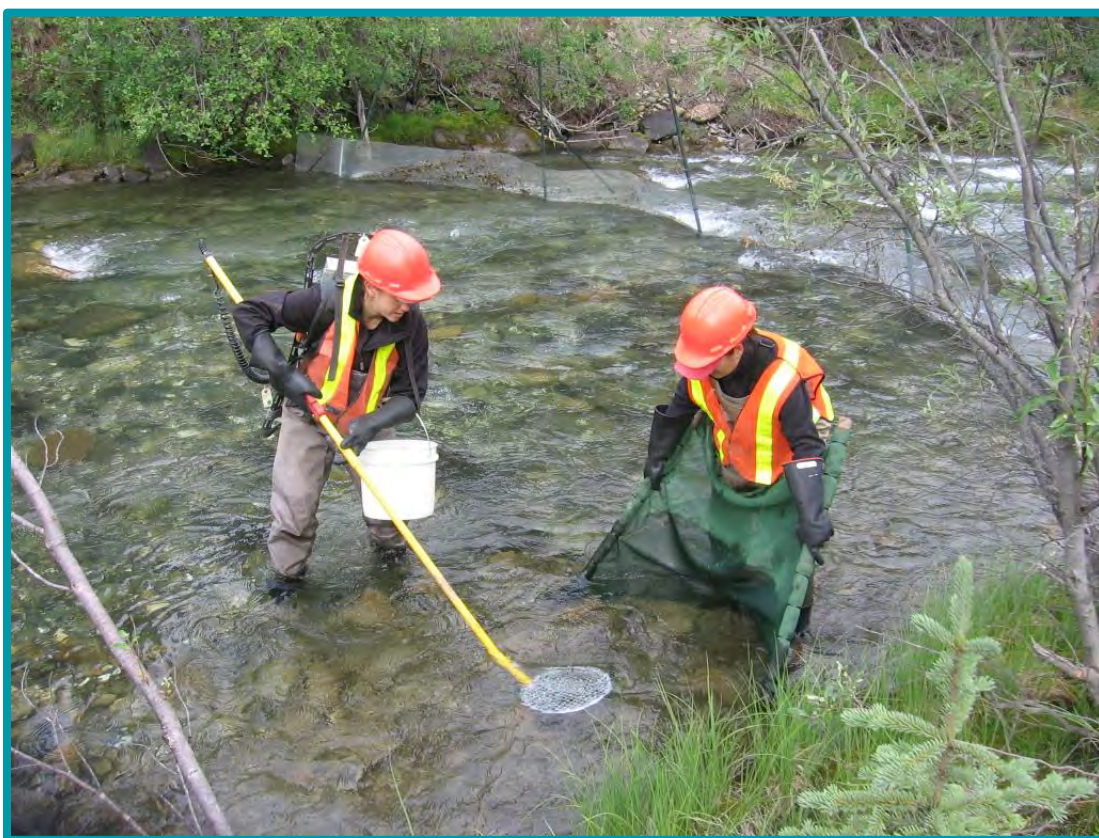
2.3.2-01 A fish salvage operation. A section of the stream was netted off and fish were collected from the isolated area by means of electroshocking. The electroshocking unit is on the back of the person on the left and the yellow pole is the shocking probe. The person on the right is helping retrieve the fish, which are only stunned for a fraction of a second so they need to be caught quickly.
