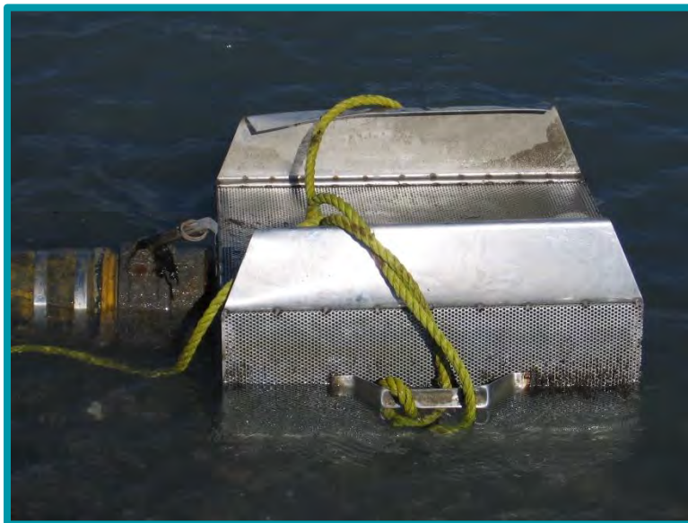
2.3.1-01 A typical fish screen for a 4" to 5" pump, fitted with correct screen size.
