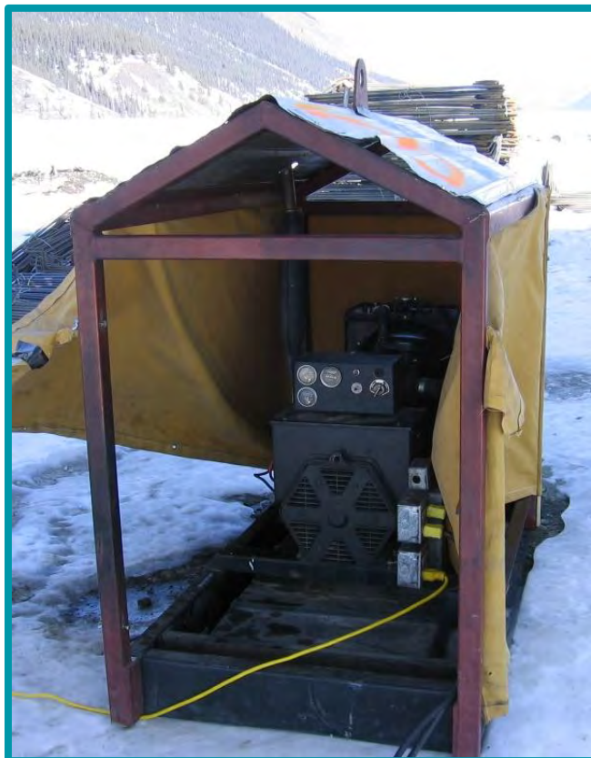
2.2.1-01 A generator properly set on a spill tray with roof and fabric to protect it from the weather.
