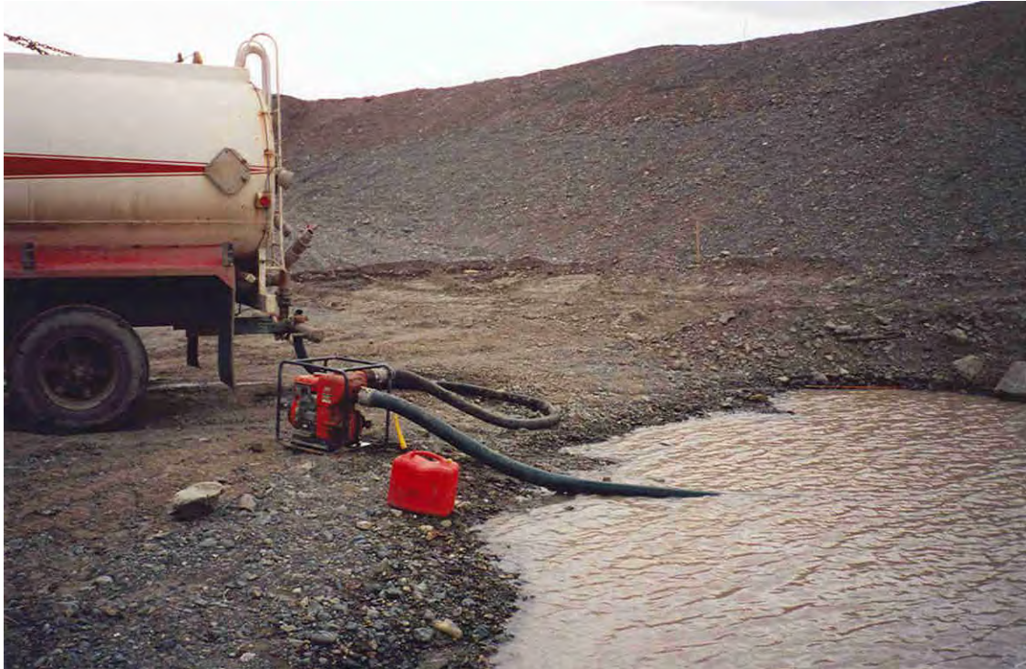
2.3.1-04 An unacceptable pump station. Water pumps need to be placed in spill trays and fuel must be stored >30m away from any water body.
