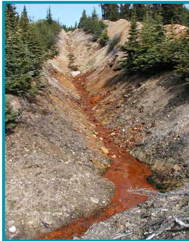
3.12-02 This exploration trench is cause for concern. The runoff is not being controlled and the colour indicates it may be contaminated with heavy metals. The straight downhill run and slope grade mean that the trench should have been reclaimed, or at least stabilized (i.e., backfilled and vegetated).
