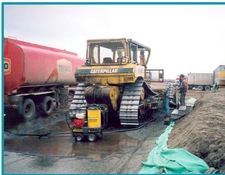
3.2-01 Pressure washing a dozer in a designated site that is lined and bermed.
