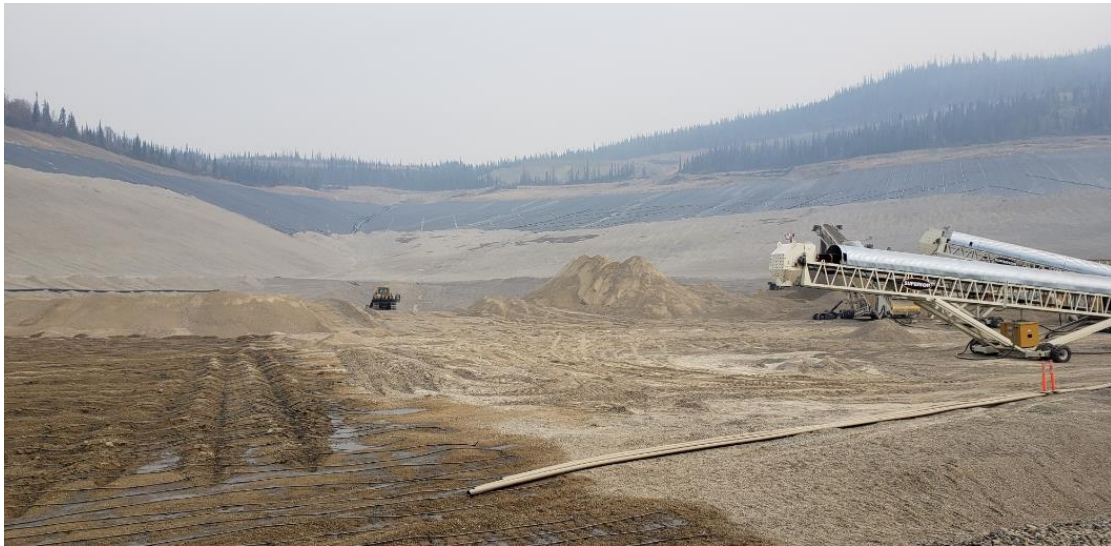
Heap leach pad with cyanide dripping from perforated tubing on left and conveyor depositing ore on right
