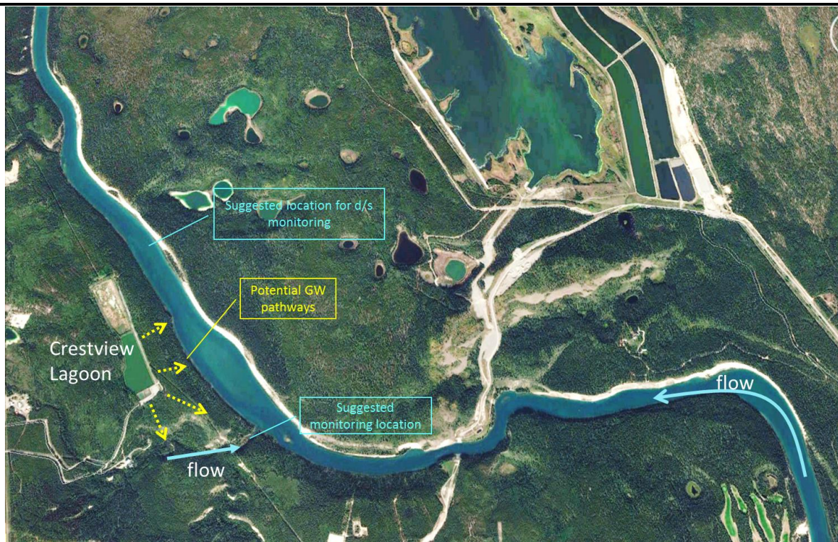
Figure 2. Suspected groundwater flow path downgradient of the Crestview Lagoon and suggested WQ monitoring location
