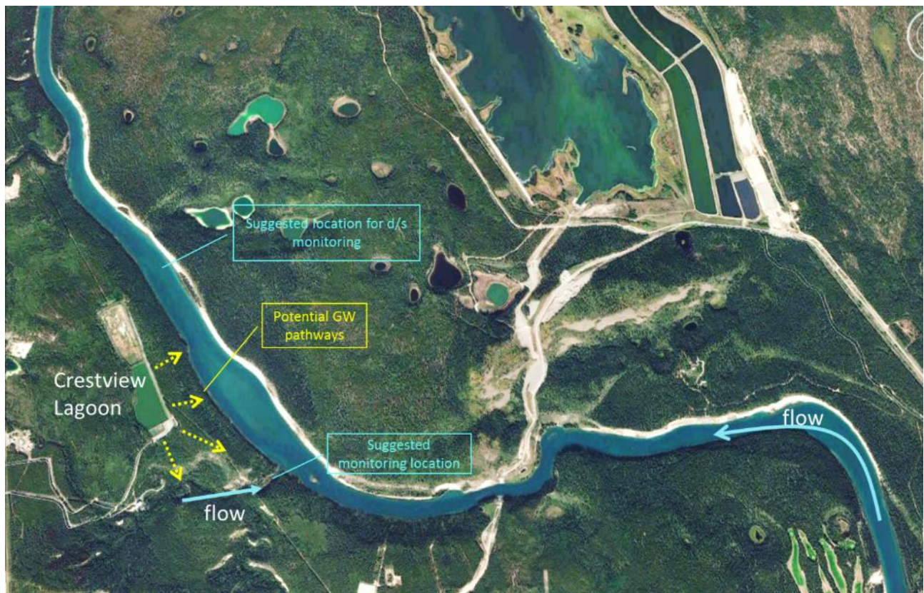
Figure 3: Suggested monitoring locations downgradient of the Crestview facility
