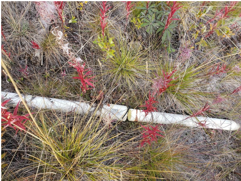
Photo 14. Station BC-70. Test cover lysimeter piping disconnected.
