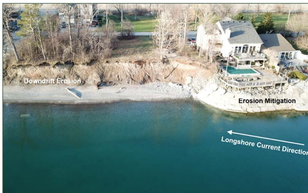
Photo 4-1. Pronounced lakeshore erosion downdrift of localized erosion mitigation on Lake Ontario (photo credit: SJL).
