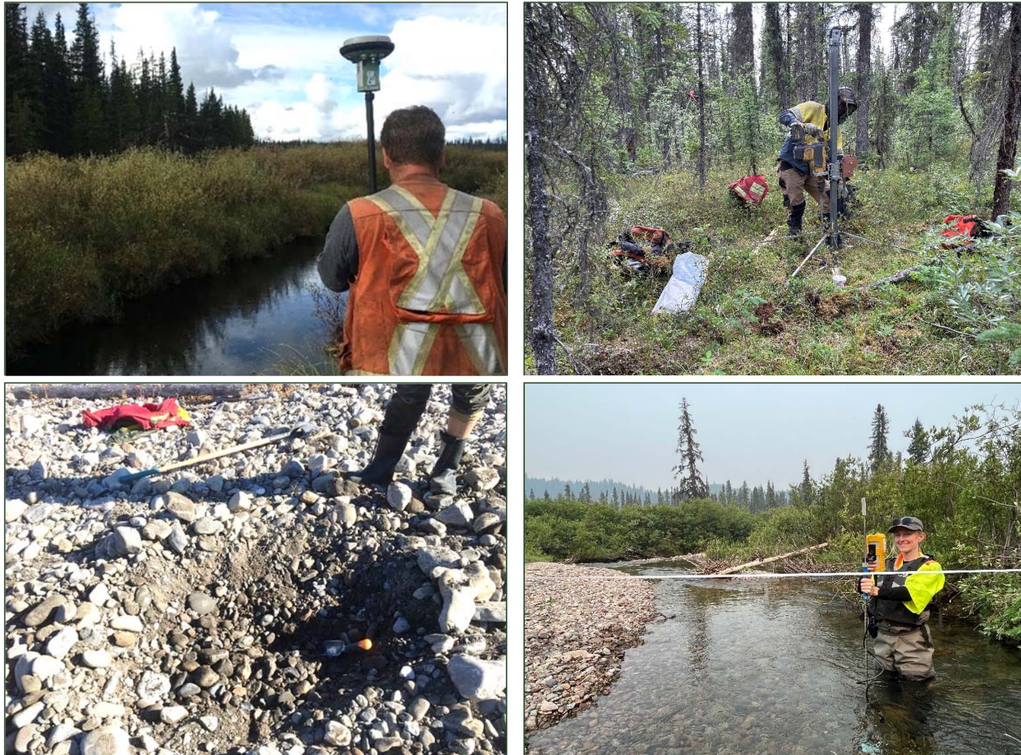
Photo 3-2. Examples of common field investigations to support detailed erosion assessments. Top left: topographic survey along a creek using an RTK GPS. Top right: shallow drilling to characterize permafrost and soil conditions. Bottom left: observation and measurements of surface and sub-surface sediments on the bed of a watercourse. Bottom right: measurement of channel hydraulics using a flow meter. All photos courtesy of SLR.
