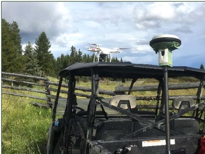
Photo 3-3. Examples of erosion monitoring. Top left: camera and staff gauge monitoring aufeis upstream of culverts (photo credit: Benoit Turcotte). Top right: monumented stakes incrementally track river migration (photo credit: Benoit Turcotte). Bottom left: UAV and RTK GPS surveys document geomorphic change (photo credit: SLR). Bottom right: meteorological thresholds (e.g., wind) can identify when lakeshore erosion may occur (photo credit: SLR).
