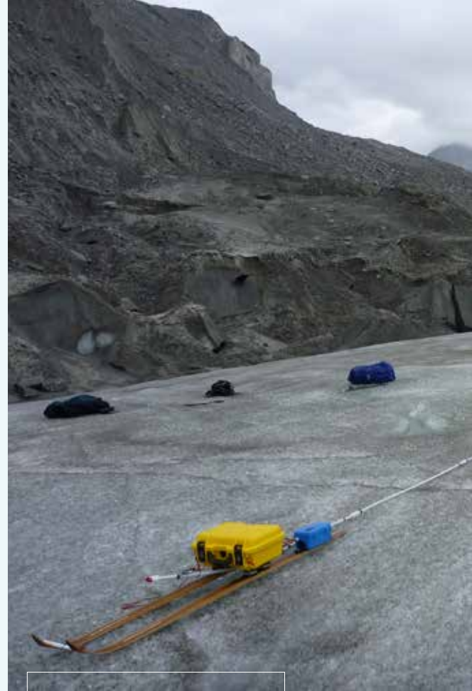
Researchers use a dual frequency penetrating radar on the Fantail Glacier to determine ice mass.
