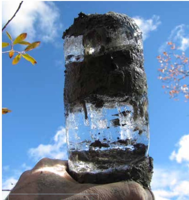
Permafrost core held up to the sky. (Yukon Research Centre, 2013)
